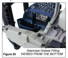
Top off gearcase grease level by using a lever-type grease gun to force 1–2 strokes of high quality lithium-based grease through the gearcase grease fitting.
